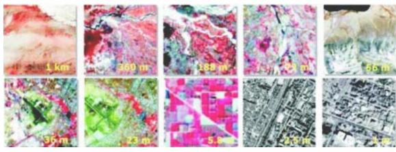
Fig. 5.2: Spatial variations of remote sensing data. Note the variations in resolution from 1 km till 1 m, in the series of photographs. The photograph taken from 1 km shows lesser details as compared to that at 1m (source: Navalgund et. al, 2007)
