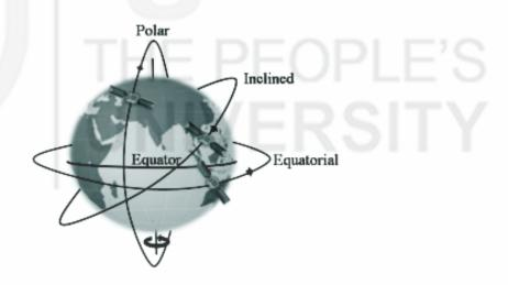
Fig. 4.2: Schematics showing three types of orbits i.e. equatorial, polar and inclined orbits
