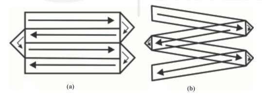
Fig. 6.9: (a) Scan line corrector mode of Landsat-7 and (b) failure of SLC (source: www.landsat.usgs.gov)
