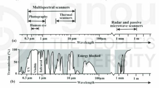
Fig. 4.8: Atmospheric transmission and the wavebands of common remote sensing systems; (a) Remote sensing scanners, and (b) atmospheric transmittance
