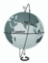
Fig. 4.5: Schematics showing the polar orbit
