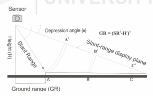
Fig. 5.13: Relationship between slant range resolution and ground range resolution (source: Gonzalez and Woods, 2002)
