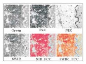
Fig. 5.6: Spectral variations of remote sensing data (source: Navalgund et. al, 2007). NIR – near infrared, SWIR – shortwave infrared, NIR FCC – near infrared false colour composite and SWIR FCC – shortwave infrared false colour composite
