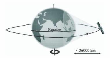
Fig. 4.4: Schematics showing the geosynchronous orbit
