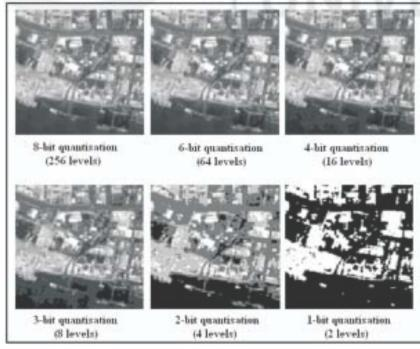
Fig. 5.7: Images showing the effect of degrading the radiometric resolution (source: www.crisp.nus.edu.sg/~research/tutorial/image.htm)
