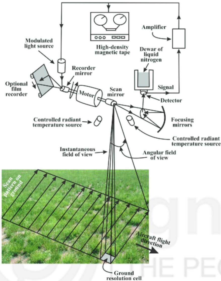
Fig. 4.12 : Schematic representation of thermal infrared scanner (modified from Sabins, 1986)
