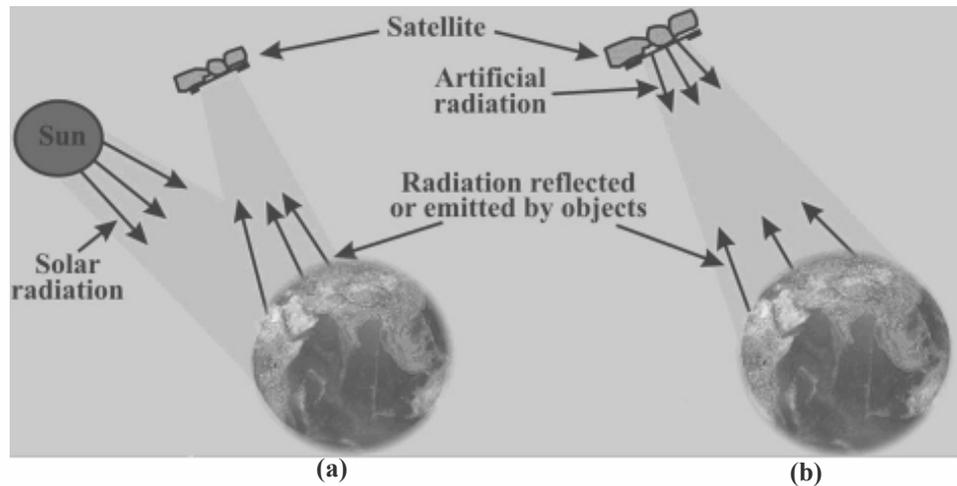
Fig. 4.7: Schematics showing the functional mechanism of (a) passive and (b) active sensors
