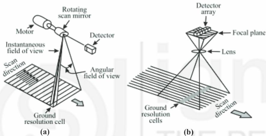
Fig. 4.9: Schematics showing sensor's scanning modes. (a) across-track mode; and (b) along-track mode (redrawn from Sabins, 1986)
