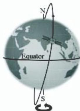
Fig. 4.5: Schematics showing the polar orbit
