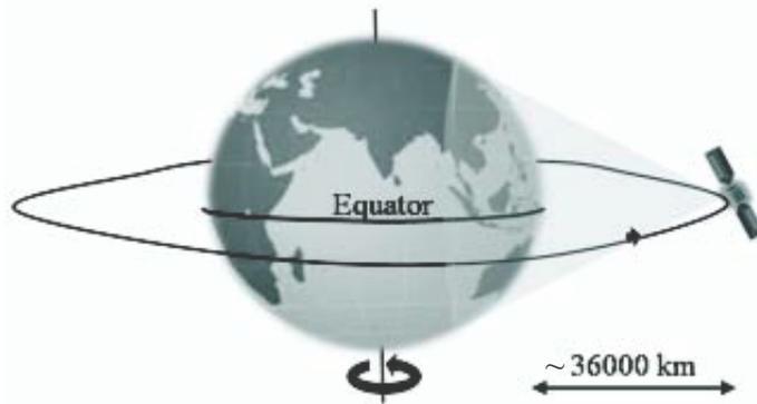
Fig. 4.4: Schematics showing the geosynchronous orbit
