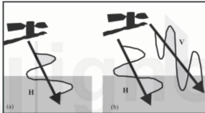
Fig. 6.10: (a) Horizontal polarisation in RADARSAT-1 and (b) both horizontal and vertical polarisation in RADARSAT-2. H – horizontal and V – vertical (source: www.asc-csa.gc.ca)
