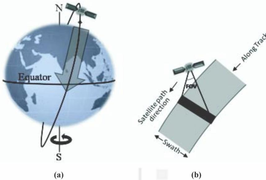
**Fig. 4.3: Schematics showing the concepts of swath and Field of View (FOV). (a) Satellite imaging a strip of land (i.e. swath) on its descending pass; (b) showing relation between FOV and swath**
