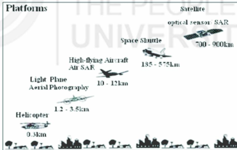
Fig. 4.1: Remote sensing platforms
