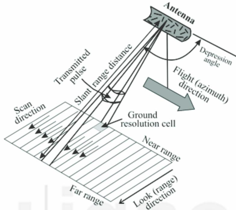
Fig. 4.11: Side looking scanning system (modified from Sabins, 1986)
