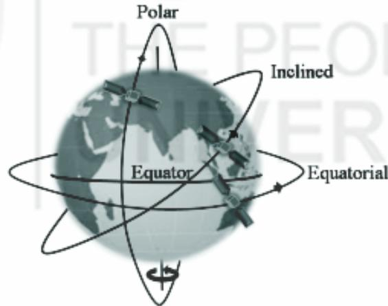
**Fig. 4.2: Schematics showing three types of orbits i.e. equatorial, polar and inclined orbits**
