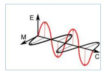
Figure: Electric and Magnetic vectors of an electromagnetic wave
